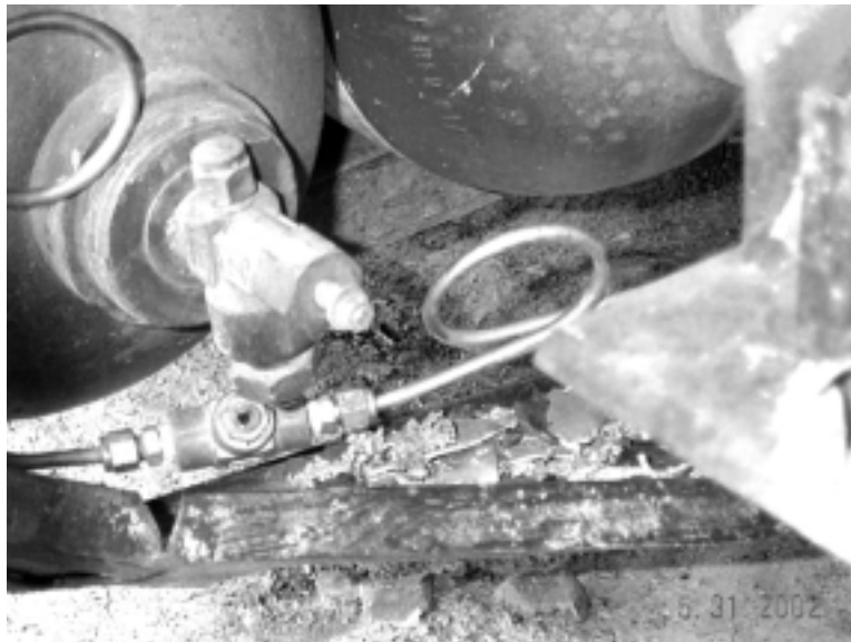
Figure 1: Cylinder valve and adapter assembly from a burned bus, broken by impact with a roadside boulder
